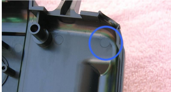
Close-up of mold mark.
